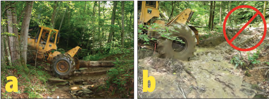
Figure 8.19. Stream with natural rock bed used as a skidder crossing (a). Fords with soft beds are not allowed and poles or other materials must be used to provide proper flotation on stream or channel beds (b).
